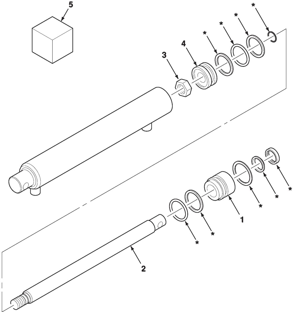
**1835 RECTANGULAR BALER****85****DECALS AND KITS****PICKUP HYDRAULIC CYLINDER ASM. (ENERGY)****(700726495 HYDRAULIC CYLINDER ASSEMBLY)**
